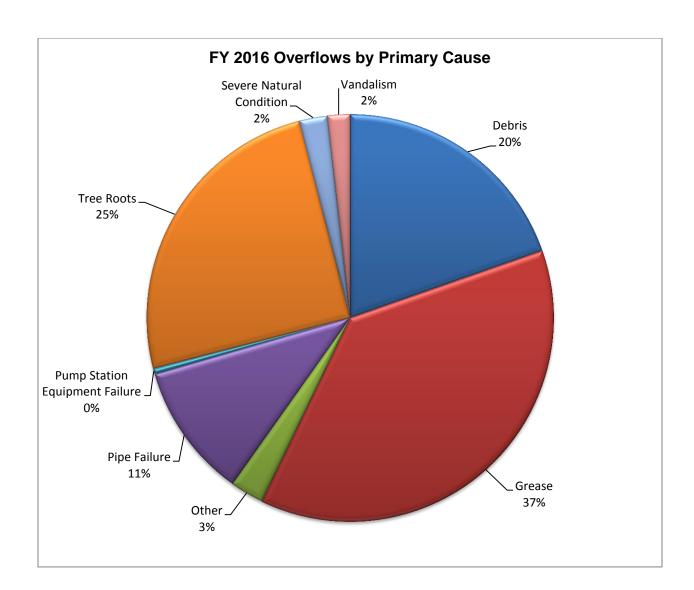
Grease and other blockages that lead to sewer overflows are cleared by CLTWater crews, using various cleaning methods, including mechanical rodders and truck-mounted water jets. If damaged pipe or other infrastructure is discovered it is repaired. The spilled wastewater can sometimes be captured and pumped back into the sewer system.
